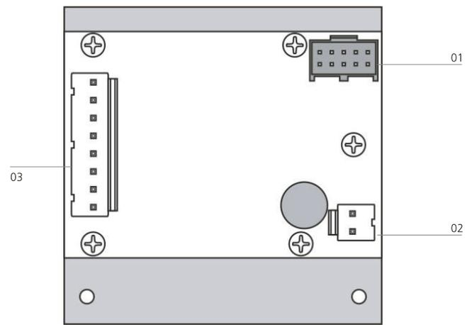
01. Input/Output Signal / External Analog Input Connector
